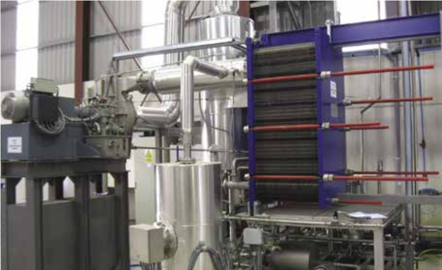
Mechanical vapour recompression system to concentrate effluent. Steam consumption reduced to zero.
