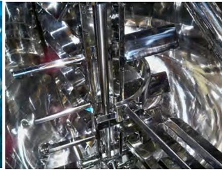
Personal care industry: toothpaste tank after 6 minutes of rotary jet head wash cycle.
