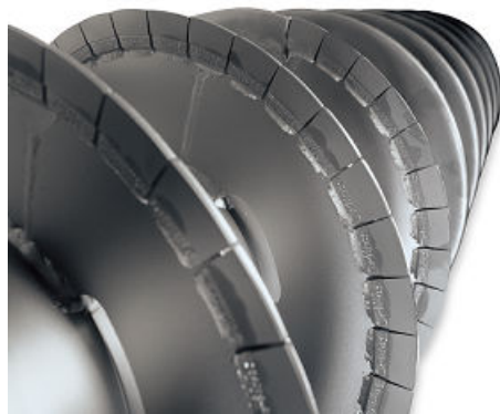
Figure 2. CDNX 300, 400, 500, 700 Example of upgraded Conveyor wear protection
